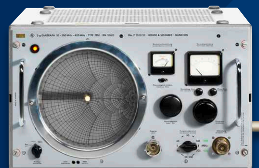
Fig. 5: The world's first vector network analyzer (1950).
