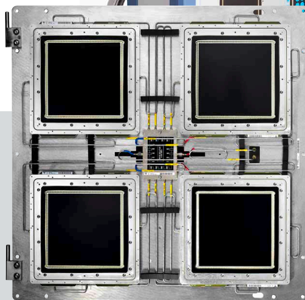
Fig. 4: Inner workings of the R&S®QPS100: signals from four antenna clusters converge at a splitter. Every cluster conceals 94 transmit and 94 receive antennas. An R&S®QPS100 consists of a total of 32 clusters.
