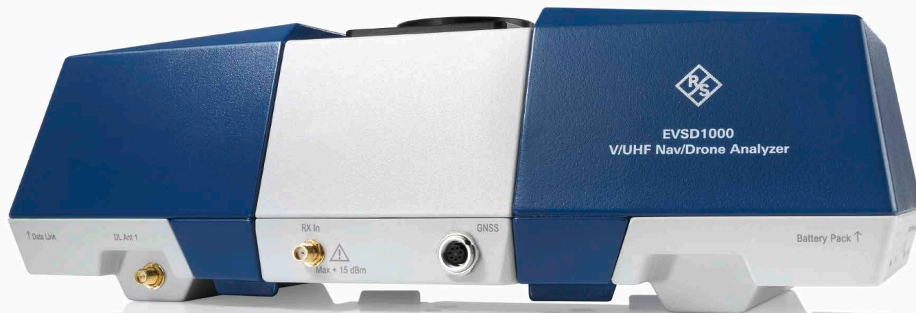
Fig. 2: The R&S®EVSD1000 VHF/UHF nav/drone analyzer is a signal level and modulation analyzer for fully ICAO-compliant, highly accurate measurement of instrument landing systems (ILS), ground-based augmentation systems (GBAS), and VHF omnirange (VOR) ground stations. It also combines many other functions in a single device, including spectrum, audio and time-domain analysis.
