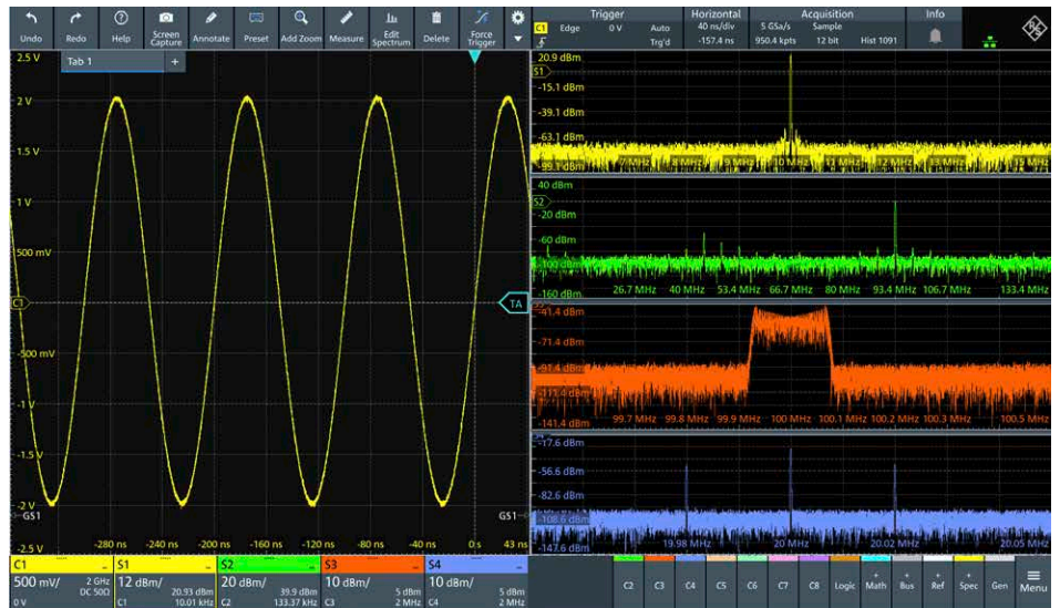
Fig. 1: A normal sine signal can conceal many spectral elements. The four simultaneous spectra shown here can be set at different spans and ranges to examine various frequency details.
