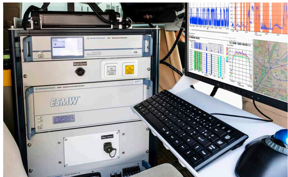
Fig. 3: The R&S®ESMW mounted in a 19-inch rack in a measurement vehicle.
