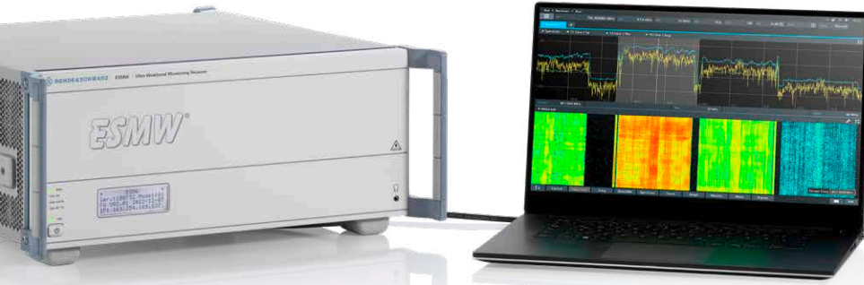
Fig. 2: The R&S®ESMW is designed for remote control from a laptop or tablet and does not need a display. The R&S®ESMW GUI is included in the scope of delivery.
