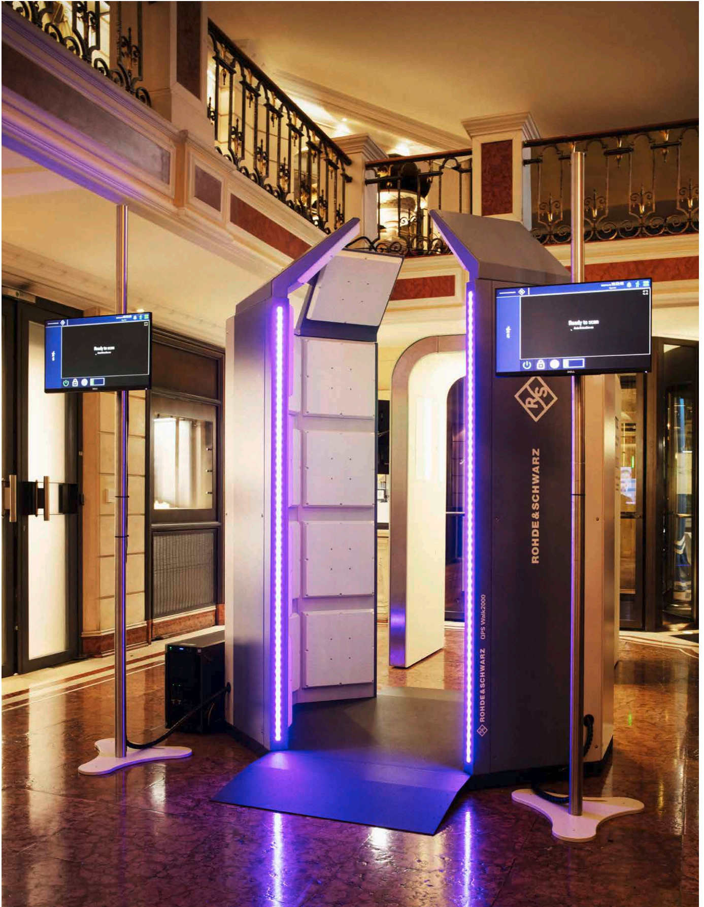
Fig. 8: The R&S®QPS Walk2000 is shown here in a photo from the Munich Security Conference in 2023. It scans while the person is walking through – without the usual brief pause inside the machine. Moreover, the outer layer of clothing does not need to be removed.
