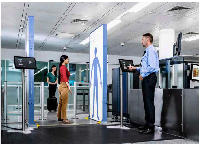
Fig. 6: The R&S®QPS201 is the latest model in the scanner family that uses the frequency range from 70 GHz to 80 GHz. The refined system design includes features like slimmed down panels.
